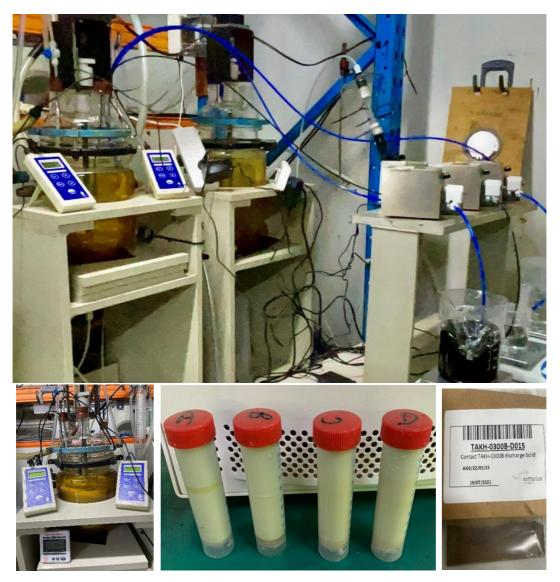
Collage 1 - NCM811 Precursor - Batch Precipitation Test
